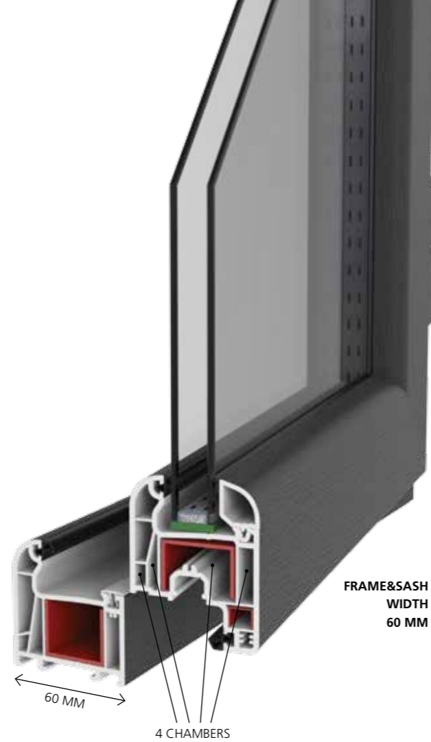
Window Heat Flow Diagram U_f: 1,46 \text{ W/m}^2 \text{ °K} U_w: 1,63 \text{ W/m}^2 \text{ °K}
